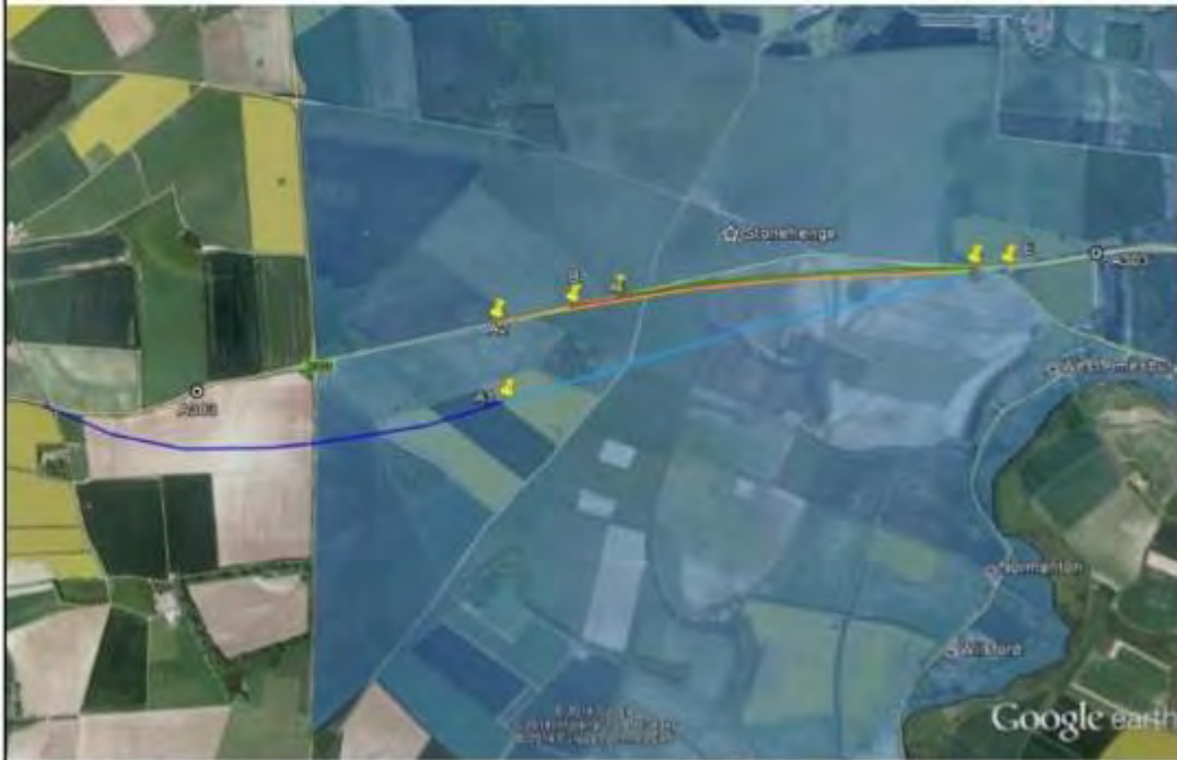
Fig. 2 Location map of the 4 different A303 tunnel options from the Snasha/1 & Young report, fig. 3, e, 28.
